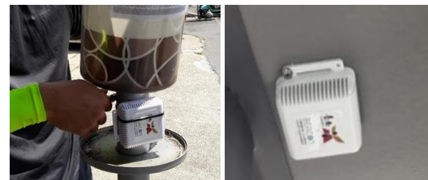
Beacons onboard and at bus stops
